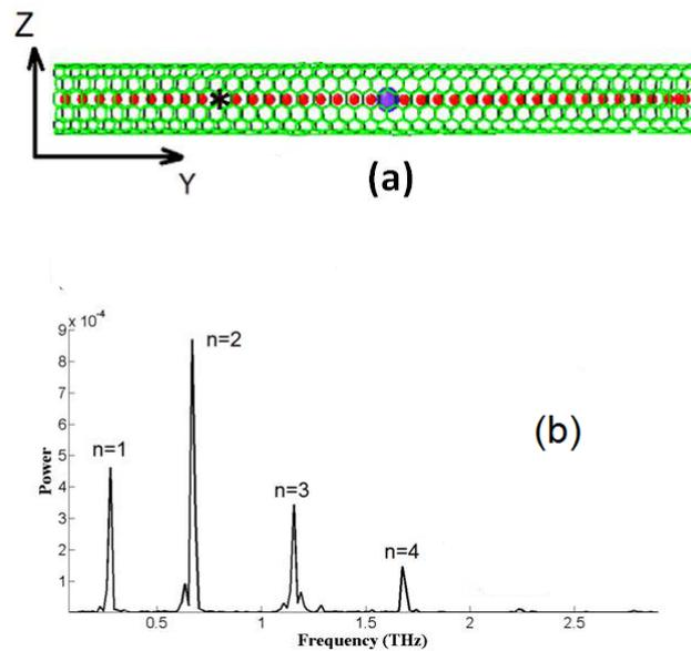
**Figure 3.** (a) Single Walled Carbon Nanotube (green), with the CA made up of the centers of mass of each period of the nanotube as (red) spheres inside the nanotube, and a (blue) large atom to indicate its CM. The \* marks one place where all the first 4 modes have finite amplitude; (b) FFT analysis of the first four thermal vibrational modes ( $n=1-4$ ) in the Z direction at this point at 300K, under doubly clamped conditions.
