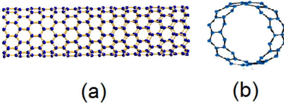
**Figure 2.** (a) (12,0) zigzag SWCNT; (b) a single period.
