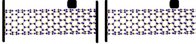
**Figure 1.** SWCNT with attached mass in a bridged configuration at left and a cantilevered configuration at right.
