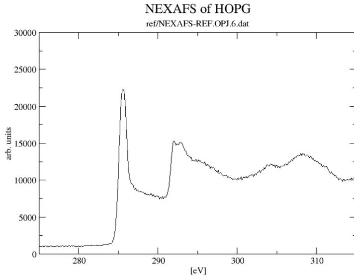
Figure 4. NEXAFS (arbitrary units) as a function of energy in eV for HOPG
