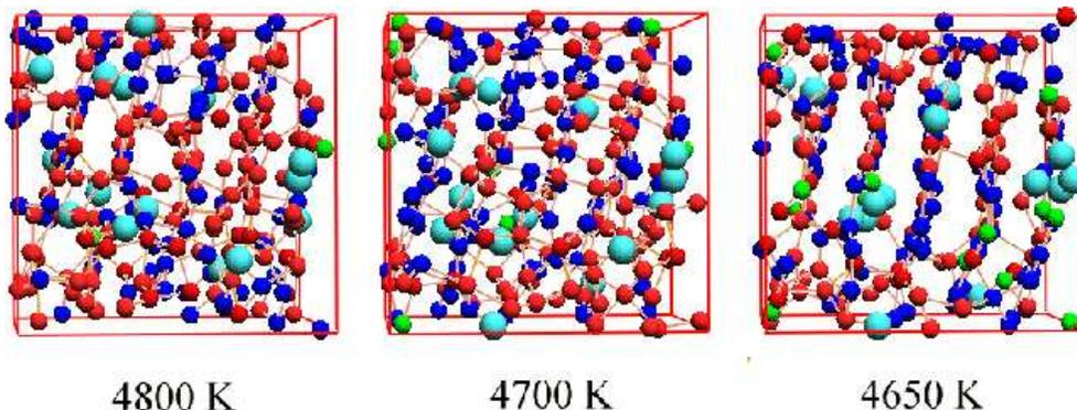
Figure 1: Snapshots of AViz visualization of hydrogenated liquid carbon at 3.9g/cc pressure with 15 H atoms during cooling. Red atoms represent 4-fold coordinated C atoms, blue represents 3-fold and green represents 2-fold coordinated C atoms. The large light-blue balls represent H atoms.
