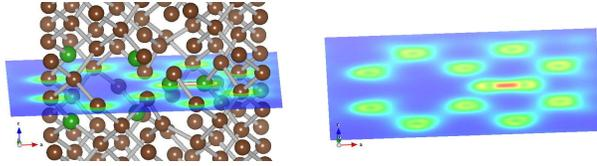
Figure 7: 2 views of the 49th frame sample showing its electronic density from VASP/VESTA. The green atoms are the 3-fold coordinated ones and in the electronic density slice red indicates the highest density, blue the lowest.
