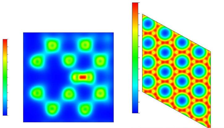
Figure 8: A view of the 49th frame sample showing its electronic density from VASP/VESTA from above compared with a  $sp^2$  bond in graphite.
