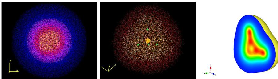
Figure 3: Electronic density of a methane molecule calculated/visualized with GAMESS/AViz, the same image stripped of the lowest densities and a methane molecule cut in the middle calculated/visualized with VASP/VESTA. Atoms are indicated by small squares(AViz) and electronic density ranges from orange (most dense) through red and pink to blue (least dense) in AViz and red to blue via green in VESTA.
