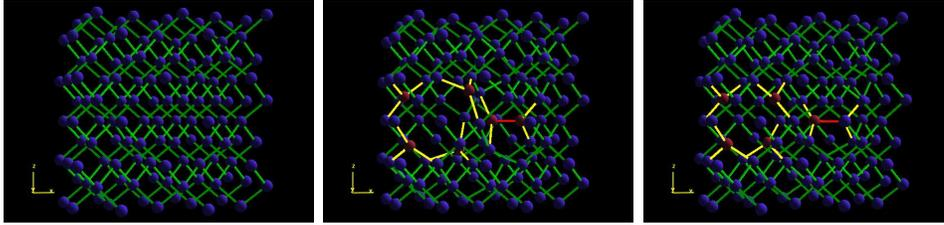
Figure 6: AViz visualization of atomic configurations of initial diamond sample, 49th out of 250 frames, and final state. Blue atoms are 4-fold coordinated, red 3-fold coordinated, bonds between two 3-fold coordinated atoms are drawn in red and bonds between a 3-fold and a 4-fold atom in yellow.
